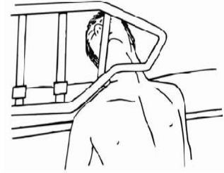
Entrapment under the bed rail at the ends of the bed rail
