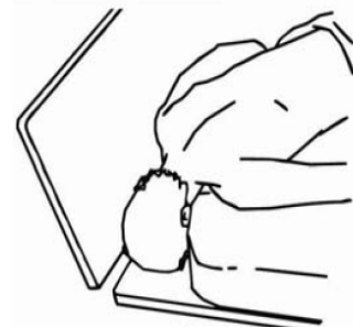
Entrapment between the head or foot board and the end of the mattress
