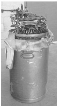
Liquid Oxygen Reservoir — After a Fire
