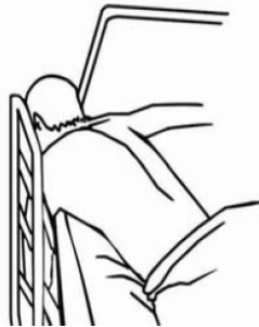
Entrapment between the end of the rail and the side edge of the head board or foot board
